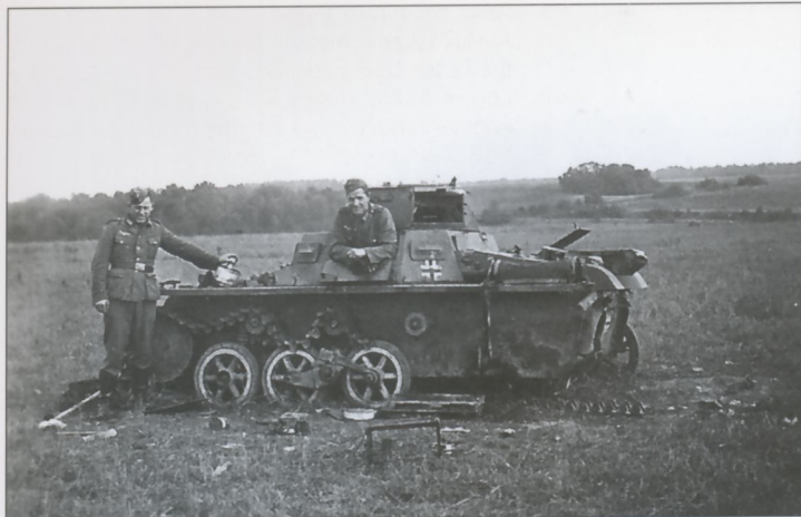
A pair of German Heer (army) soldiers takes time from exploring this destroyed Pz.Kpfw.I Ausf.A to pose for a souvenir photograph. The Panzer has shed much of its suspension system and tracks and has suffered a rupture in the armor at the lower rear hull area. Likewise, the gun mantle and both MG13ks are missing. The Panzer has additional armor fitted to the rear deck.
