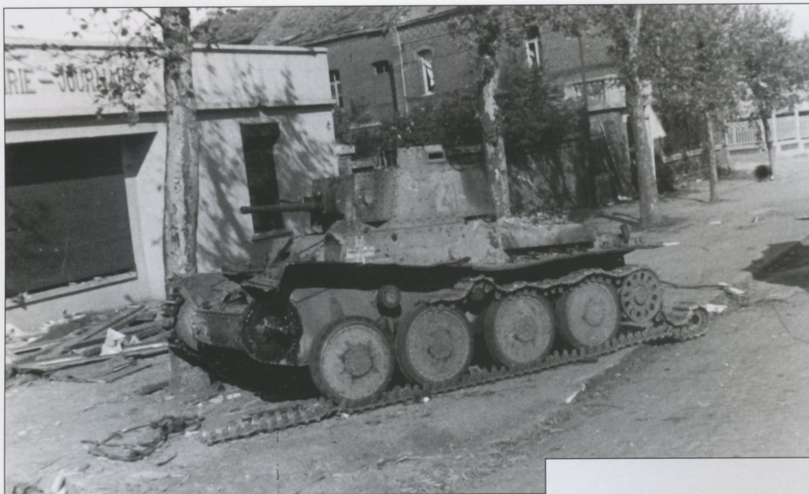
This Pz.Kpfw.38(t) Ausf.B, C or D lies destroyed and partially stripped somewhere in France during the 1940 campaign. Note the remnants of a three-digit Tac number on the turret side wall and a white-outline Balkenkreuz on the near-side superstructure. The tracks have been disconnected and the drive sprocket has been removed.
