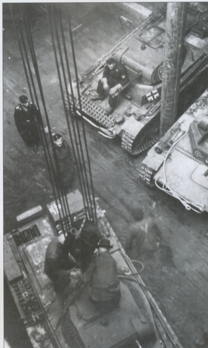
This trio of Pz.Kpfw.IIs (Ausf.A, B or C) was photographed while being loaded onto (or un-loaded from) the hold of a transport ship. The Panzer at upper right carries markings identifying it as belonging to Pz.Abt.z.b.V.40, which saw action during the invasion of Norway in April of 1940. All appear to have parts of the up-grade package, including Zusatzpanzer (appliqué armor panels) on the superstructure front and the turret front and Vorpanzer (spaced armor) on the bow. A Notek black-out driving head-lamp has been mounted onto the glacis plate Vorpanzer, instead of the more common position on the port-side track-guards.
