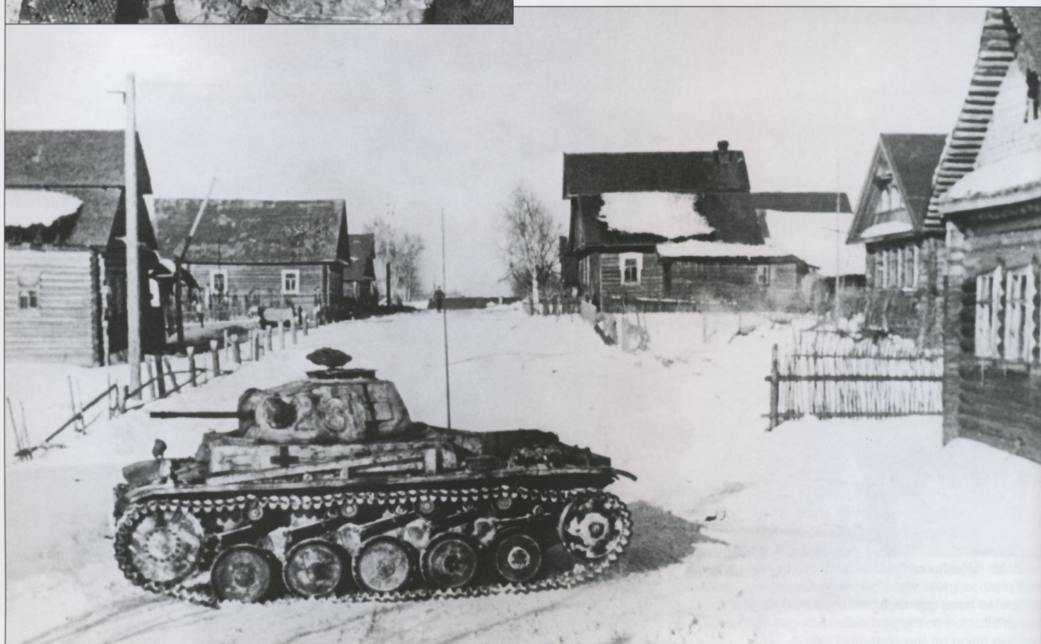
These two images provide two angles of the same Pz.Kpfw.II Ausf.F. It is identified as an Ausf.F by the straight superstructure front plate, the retention of the five road-wheels with spring bundles for the suspension, the return rollers, track links with pairs of edge-mounted guide horns, drive sprocket with single toothed ring and later style idler wheel. The head-on view shows battle damage on the starboard track-guard and stowage locker, while the side view shows a Tac number on the turret, probably 231.
