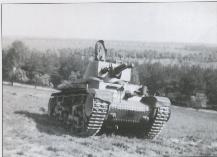
This non-descript Pz.Kpfw.35(t) moves along a hill-side, probably during a training exercise. A registration number, possibly 13476, is painted in black, low on the bow plate. Note the cover over the muzzle of the 3.7cm KwK(t) and the lack of flash suppressors on both 7.92mm MG37(t)s.
