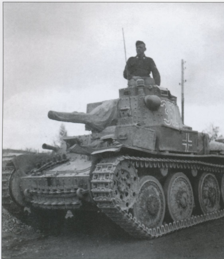
This Pz.Kpfw.38(t) Ausf. B, C or D is seen during the opening stages of Operation Barbarossa in June of 1941, as it makes its way into Stalin's Soviet Union. Note the tapered tube on the horn as well as the Notek black-out driving head-lamp on the far and near track-guards, respectively. A white-outline three-digit Tac number, 352, has been painted on the turret side wall, while a black/white Balkenkreuz national insignia is seen on the track-guard-mounted stowage locker. As all weapons are covered for protection from the ever-pervasive mid-summer dust, combat does not appear imminent.
