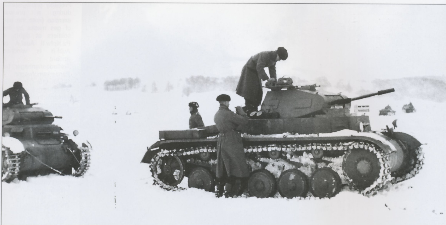
In pre-war exercises, a Pz.Kpfw.II Ausf.A or Ausf.B prepares to tow its companion through a blanket of snow. The crewmen wear their standard M1935 greatcoat over their all-black uniforms. Typical for the era, the leichte Panzer are devoid of any markings. At the estimated time this photo was taken, they would have been finished in the two-tone camouflage scheme consisting of a base of Dunkelgrau Nr.46 over-sprayed with Dunkelbraun Nr.45 in patches, so the latter color covered roughly 1/3 of the item being painted.
