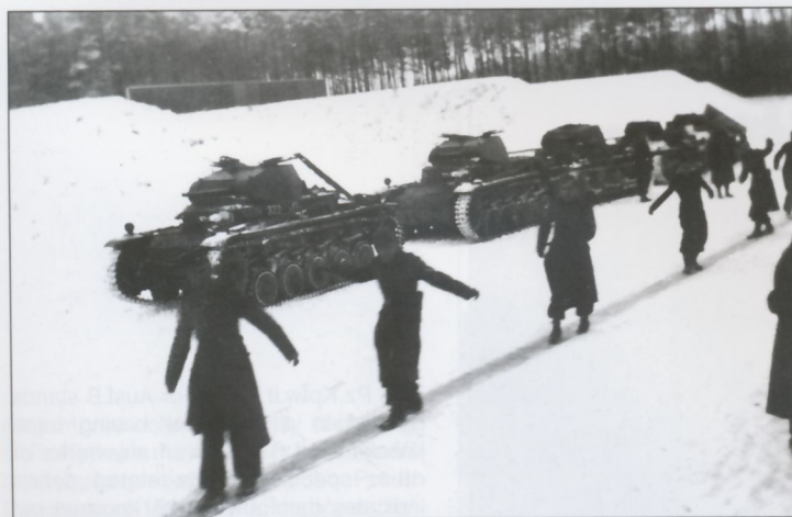
Quite probably photographed in the winter of 1939-1940, after the Balkenkreuz national insignia was ordered changed to the black/white style seen here, a Zug (platoon) of three Pz.Kpfw.II Ausf.A, B or C and a pair of Pz.Kpfw.IIs are parked in a column in this snowy setting. Note that these 3.Kompanie leichte Panzer also carry a three-digit Tac number on a rhomboid plate attached to their superstructure sides.
