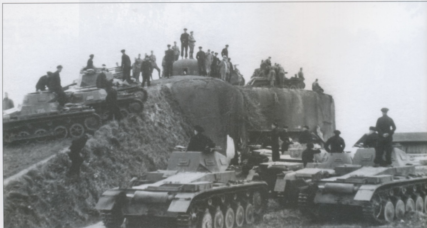
A previous photograph in this book depicted a Pz.Kpfw.I next to this bunker complex; here we see several more, joined by some Pz.Kpfw.IIs. Note the absence of the swing-out anti-aircraft machine-gun mount on the near side of both Pz.Kpfw.IIs as well as the relative lack of any visible markings, except rhomboid plates for Tac numbers.
