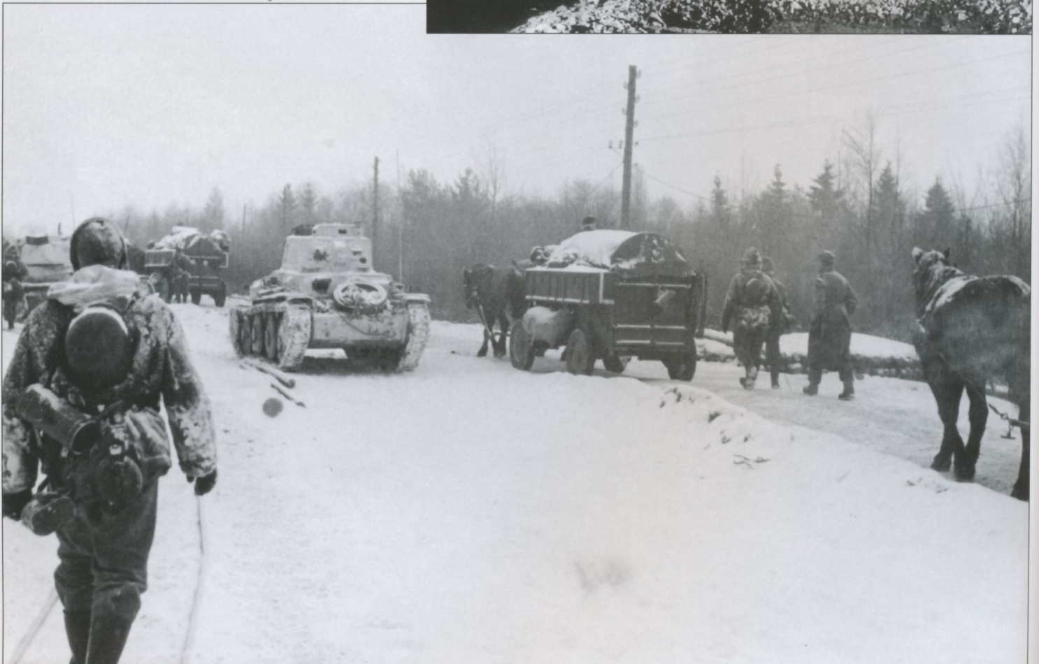
A Pz.Kpfw.38(t) Ausf.G moves along a snow-covered track somewhere on the Ostfront; the placement of the Notek black-out driving head-lamp on the glacis identifies the model. It has been white-washed for concealment against the snow and there is a dark spot on the side of the turret, which is a partial view of a Tac number. A road-wheel has been stored on the bow, with the back-side out so it acts as a stowage tray for cables and other paraphernalia.
