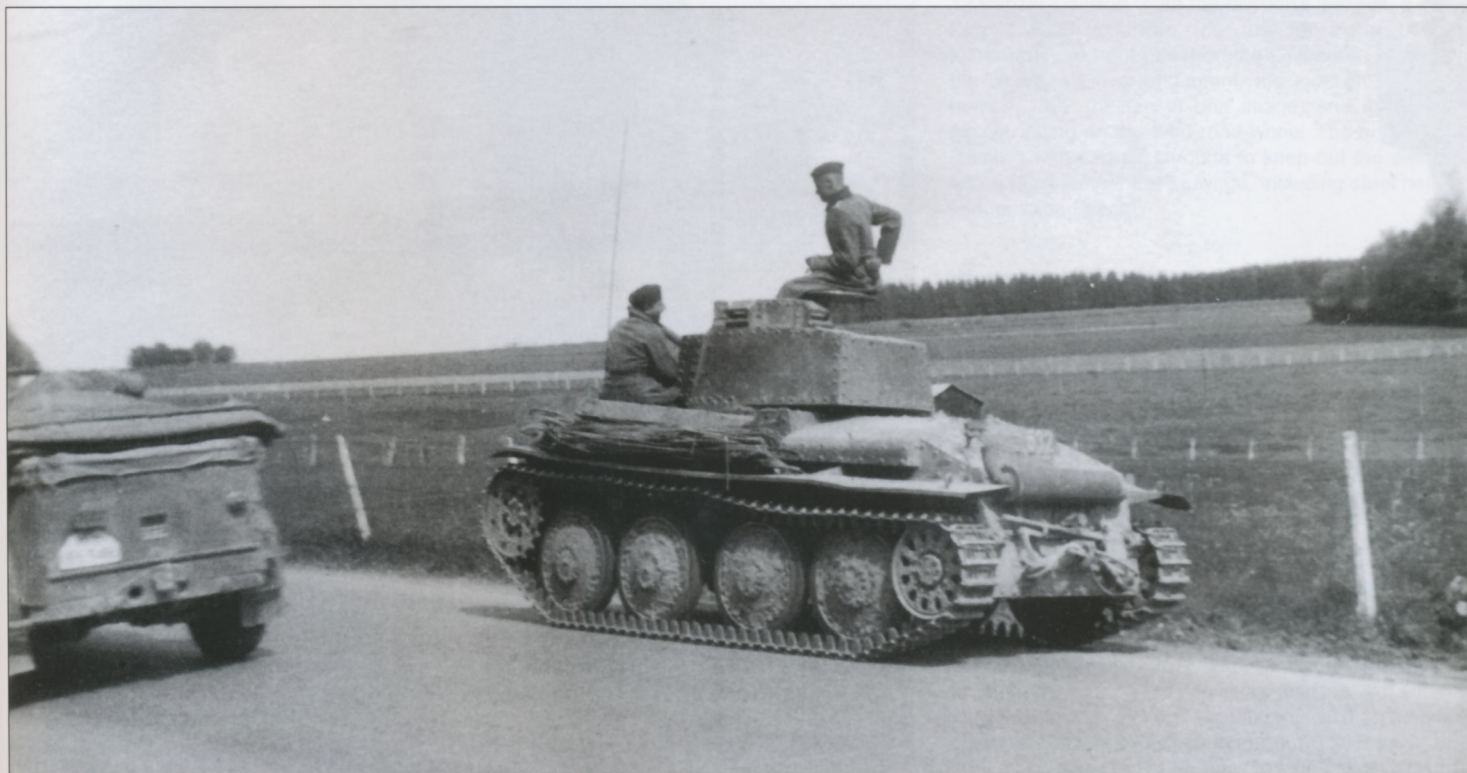
Two crew-members of this Pz.Kpfw.38(t) Ausf.B, C or D converse while their Panzer is halted on the road-side. Note the bundle of fascines on the track-guard and the re-located shovel and tow-cable, now seen on the hull rear plate. This dusty vehicle shows no markings except for a three-digit Tac marking, 532, on a rhomboid plate attached to the engine deck.
