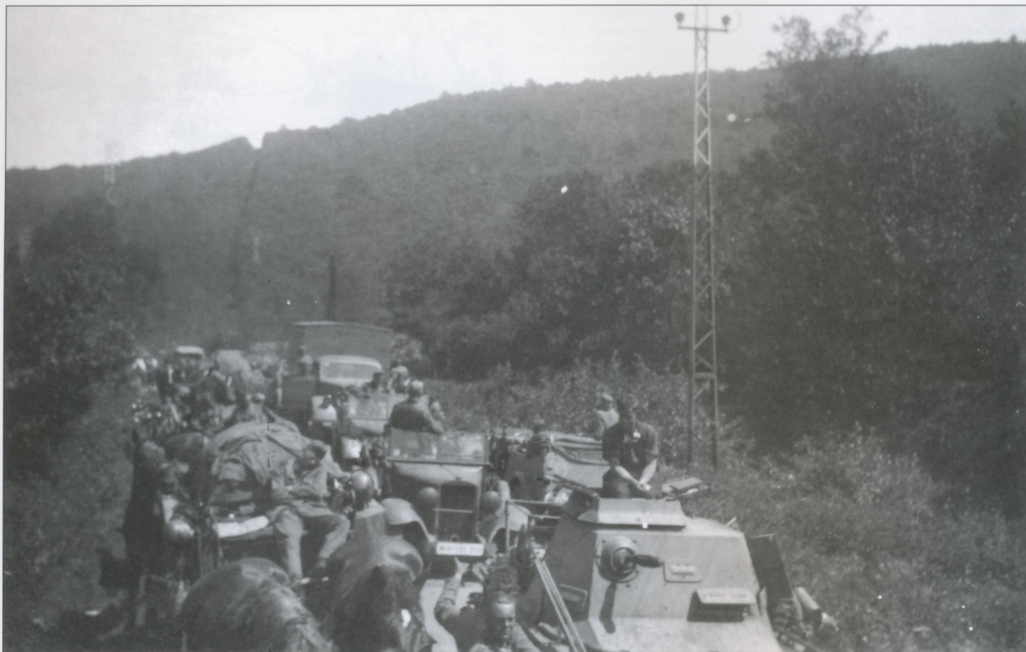
A wheeled vehicle column, most likely a divisional or regimental command unit, is led by the first main derivative of the Pz.Kpfw.I, the kleine Panzerbefehlswagen (Sd.Kfz.265). This AFV dispensed with the rotating machine-gun-armed turret for a heightened, fixed superstructure upon which was mounted an observation cupola; initial versions did not have a cupola. It was crewed by three men and carried various radios such as the Fu.2 and Fu.6.
