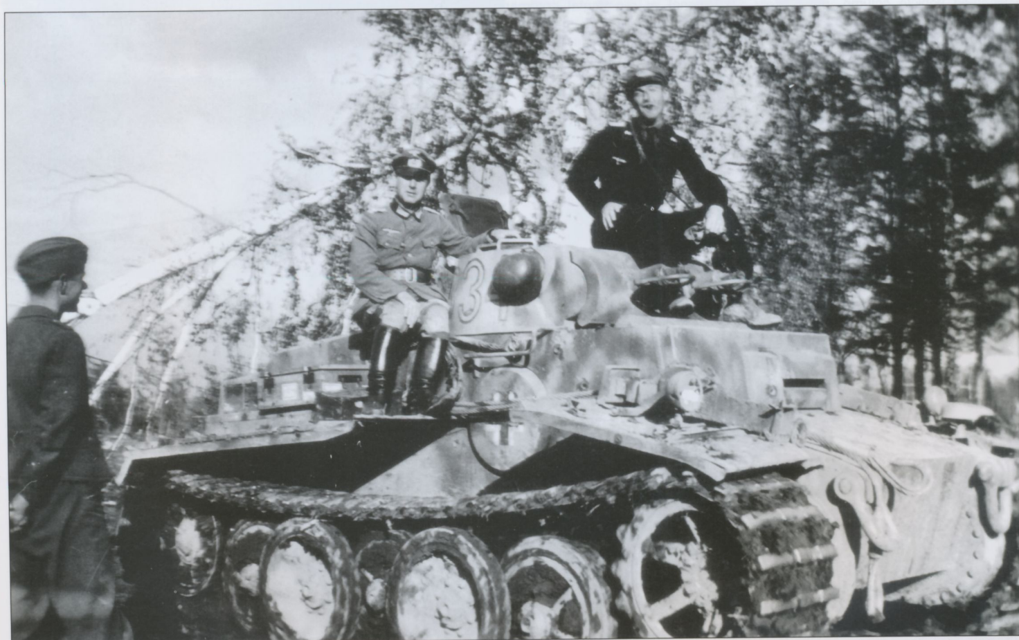
The ultimate Pz.Kpfw.I was the Ausf.F, seen here deployed with Panzer-Abteilung z.b.V.66 on the Ostfront in 1942. This Panzer featured interleaved road-wheels mounted on torsion bar suspension units and armor plate of up to 80mm in thickness on the bow plate, superstructure front plate and gun mantle. Rather overweight at 21 metric tons for the armament carried (2 x 7.92mm MG34s) it represented a design dead-end at a time when Germany could little afford such a luxury.
