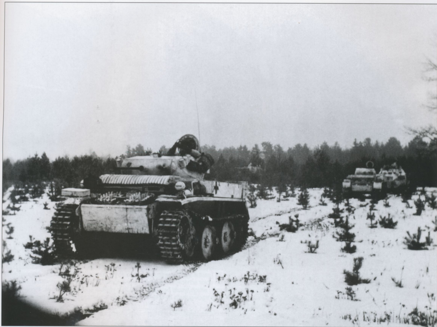
Seen moving across a snowy Ostfront landscape, this Panzerspähwagen II (2cm) (Sd.Kfz.123) Luchs (Lynx) from 4.Panzer-Division again shows stowage arrangements and modifications typical of this unit. At this stage, the curved front mud-flaps are gone from the track-guards but the spaced plate on the bow is still retained as are the pair of triple Nebelwurfgerät (smoke candle dischargers) mounted on the front corners of the turret. Idler wheel segments are stowed on the forward edge of the superstructure and spare track links are seen on the glacis plate. The sole visible marking is the Balkenkreuz seen on the stowage locker on the near side track-guard.
