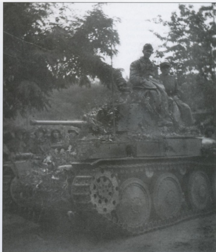
This heavily-stowed and dusty Pz.Kpfw.38(t) Ausf. G has paused on the side of the road for a photograph. It is identified as an Ausf. G by the bolt pattern on the forward edge of the turret and the single piece of 50mm armor on the front plate. A series of stowage lockers have been fitted to the near-side track guard and the Panzer has been partially covered with foliage in order to break up its outline. Note the position of the Notek black-out driving head-lamp on the edge of the glacis plate (another Ausf. G feature) and the location of the fire extinguisher on the far track-guard.
