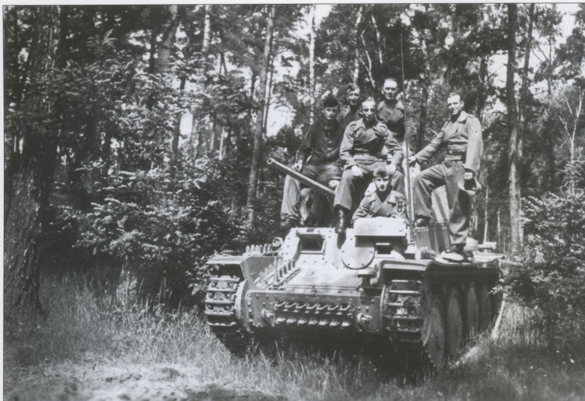
The four-man crew of this Pz.Kpfw.38(t) Ausf. B, C or D als Zugfr.Wg. (platoon commander's vehicle) pose with some friends for posterity. Note the circular plate over the radio operator's position where the 7.92mm MG37(t) has been removed to make room for additional radio gear in its stead. The Notek black-out driving head-lamp has been fitted on the port side edge of the glacis plate. Spare track links can be seen fitted to the bow and glacis plates on the standard racks, while more are seen on the starboard side track-guard.
