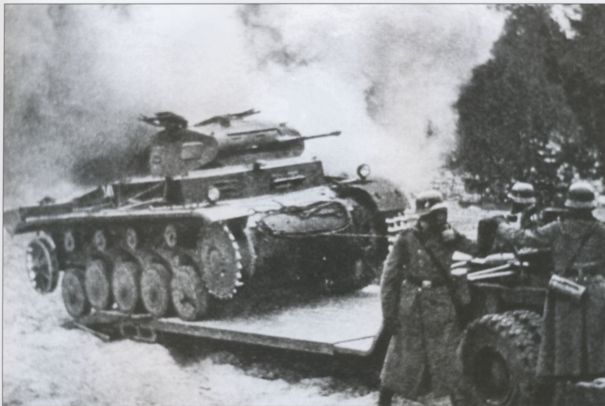
Probably photographed during a pre-war exercise (note the use of gas masks by the soldiers at right), a Pz.Kpfw.II Ausf.A or Ausf.B is winched aboard a Tiefladeananhänger für Panzerkampfwagen Sd.Ah.115. Note the cable leading from the bow of the leichte Panzer and that the tracks on the near side have been removed. The frame seen on the superstructure side plate was a mount for an anti-aircraft machine-gun, which was hinged so it could swing out away from the vehicle.
