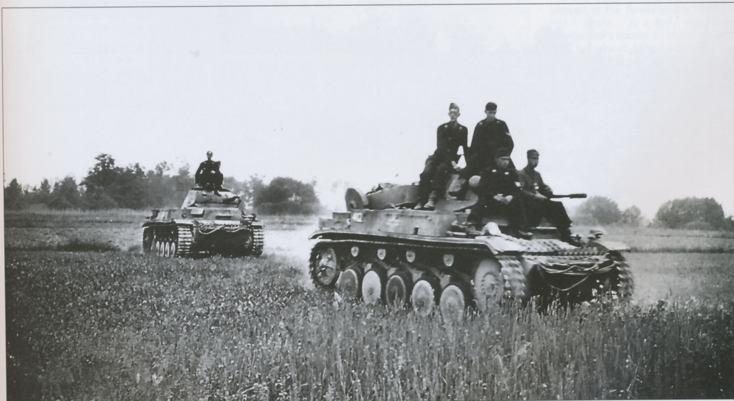
A pair of dust-covered Pz.Kpfw.IIs (Ausf.A, B or C) crosses an open field. Both have all of the requested modifications including: Notek black-out driving head-lamp on the port side track-guard, Vorpanzer (spaced armor) on the bow and Zusatzpanzerung (appliqué armor) on the turret front and superstructure front, commander's cupola with round, single-piece hatch lid and periscopes around the rim and stowage locker on the starboard side track-guard. There is a black/white Balkenkreuz national insignia on the stowage locker, and there is also a rhomboid plate attached to the stowage box behind it, with a white Tac number, possibly "402". Note the unusual, unidentified item on the near leichte Panzer's engine deck.
