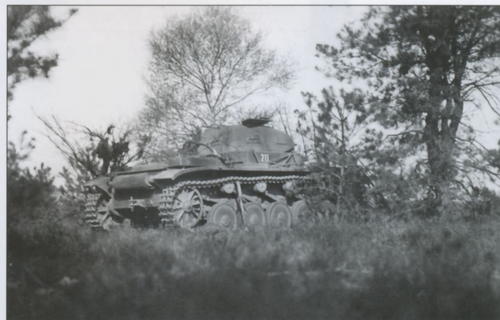
A Pz.Kpfw.II (probably an Ausf.c as indicated by the anti-aircraft machine gun mount) lurks in a tree-line, probably during pre-war exercises; note that it does not wear any form of Balkenkreuz national insignia, which was typical for that era. A white Tac number, 211, has been painted on the superstructure side plate just behind the pivoting anti-aircraft machine-gun mount. Although this leichte Panzer is fairly dusty, evidence that it is finished in the two-tone camouflage scheme of Dunkelgrau Nr.46 over-painted with Dunkelbraun Nr.45, can be seen on the turret and the rear-most stowage locker on the near-side track-guard.
