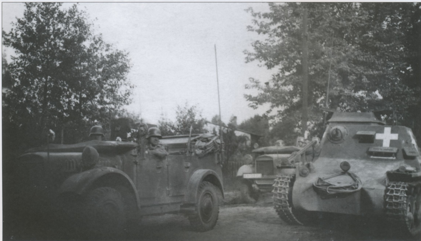
This command element from a Panzer-Division is seen on a dusty road during the Polish Campaign of September 1939. The kl.Pz.Bef.Wg. (Sd.Kfz.265) wears the thick white Balkenkreuz national insignia on all four surfaces of the superstructure, characteristic of the campaign. Next to the AFV are a pair of BMW light field cars outfitted to carry radios; in such a configuration they were designated Kfz.22.
