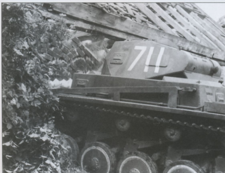
This Pz.Kpfw.II shows clear evidence of the post-July 1937 two-tone camouflage scheme of Dunkelgrau Nr.46 over-painted with Dunkelbraun Nr.45, particularly on the turret side walls. Note also the Tac numbers, 711, in white as well as the absence of any armament. This leichte Panzer has disabled itself by driving into the brick wall of a building. Finally, there appears to be an attempt made at deceiving the enemy as to the exact location of the view-port on the superstructure rear plate; note the two-tone shape painted next to it.
