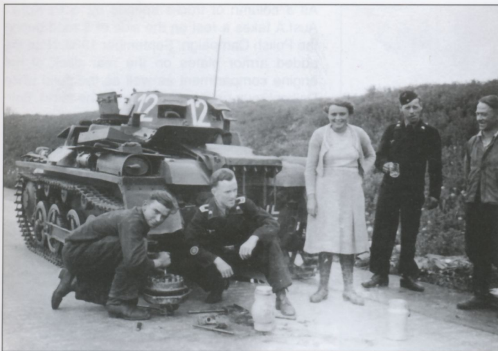
The crew of a Pz.Kpfw.I Ausf.A works on their Panzer, while a pair of locals, probably the source of the drink being held by a third soldier, stands by. This Panzer has been retrofitted with armored cowls on the rear plate and engine deck, as well as with a Nebelkerzenabwurfvorrichtung (rack to deploy smoke candles). It wears white Tac numbers, 12, on the turret in three places and is marked with a black/white Balkenkreuz low on the hull rear plate.
