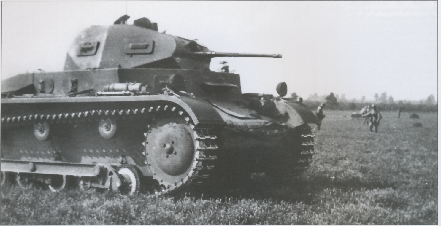
The first version of the Pz.Kpfw.II was the Ausf.a/1, a/2 and a/3 (although this particular vehicle's model type is undetermined), all of which had similar features. Identifying features from this angle include the shape of the drive sprocket hub, the style of view-port covers on the turret and the suspension system with its support girder. Note the two round armored hatch lids on the superstructure side plate, aft of the turret; these covered fuel filler caps.
