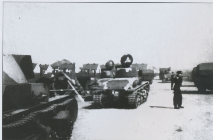
A German Panzer crewman adjusts his clothing while a trio of Pz.Kpfw. L.T.Sk.35s awaits his attention. Note that the nearest Panzer has a German vehicle jack laying on the track-guard; also of interest is the protruding stowage locker that was integrated into the front-most bogie wheel assembly. All visible Panzer wear their Czech camouflage colors, while the one in the center of the photo also retains the original five-digit registration numbers on the rear plate.
