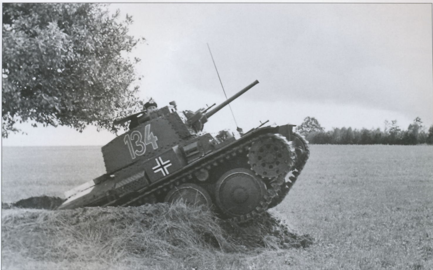
This brightly-marked and relatively clean Pz.Kpfw.38(t) Ausf.B, C or D makes its way out of its hull-down position, possibly just prior to the French Campaign in 1940. Note again the large three-digit Tac number, 134, on the side of the turret; it would again appear that the fill color is far lighter than red or black. A black/white Balkenkreuz is seen on the track-guard mounted stowage locker and there is a prominent white rectangle painted on the engine deck as an aerial recognition device.
