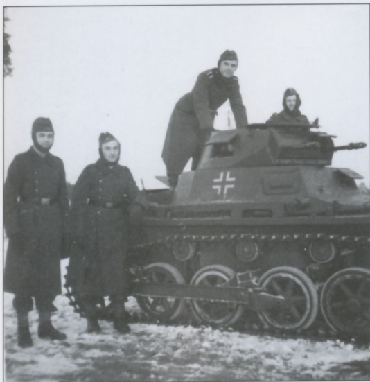
On 26 October 1939, German AFVs were ordered to use a new style of Balkenkreuz national insignia. Instead of a thick, all-white marking, the new style consisted of a black center with a thin white outline. Sometimes the black center was not applied as appears to be the case here. Otherwise, this Pz.Kpfw.I Ausf.A is in the standard configuration.
