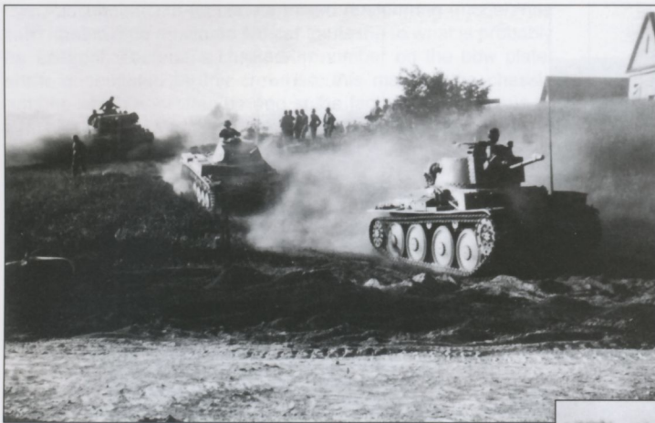
This Pz.Kpfw.38(t) Ausf. B, C or D (identified by the bolt pattern on the turret front plate for 25mm armor) raises a cloud of dust as it leads a Pz.Kpfw.II Ausf.A, B or C and a Pz.Kpfw.IV down an incline. This Panzer has not had extensive stowage modifications made to it, nor does it exhibit much in the way of extra gear hanging about; additionally, no markings are visible.
