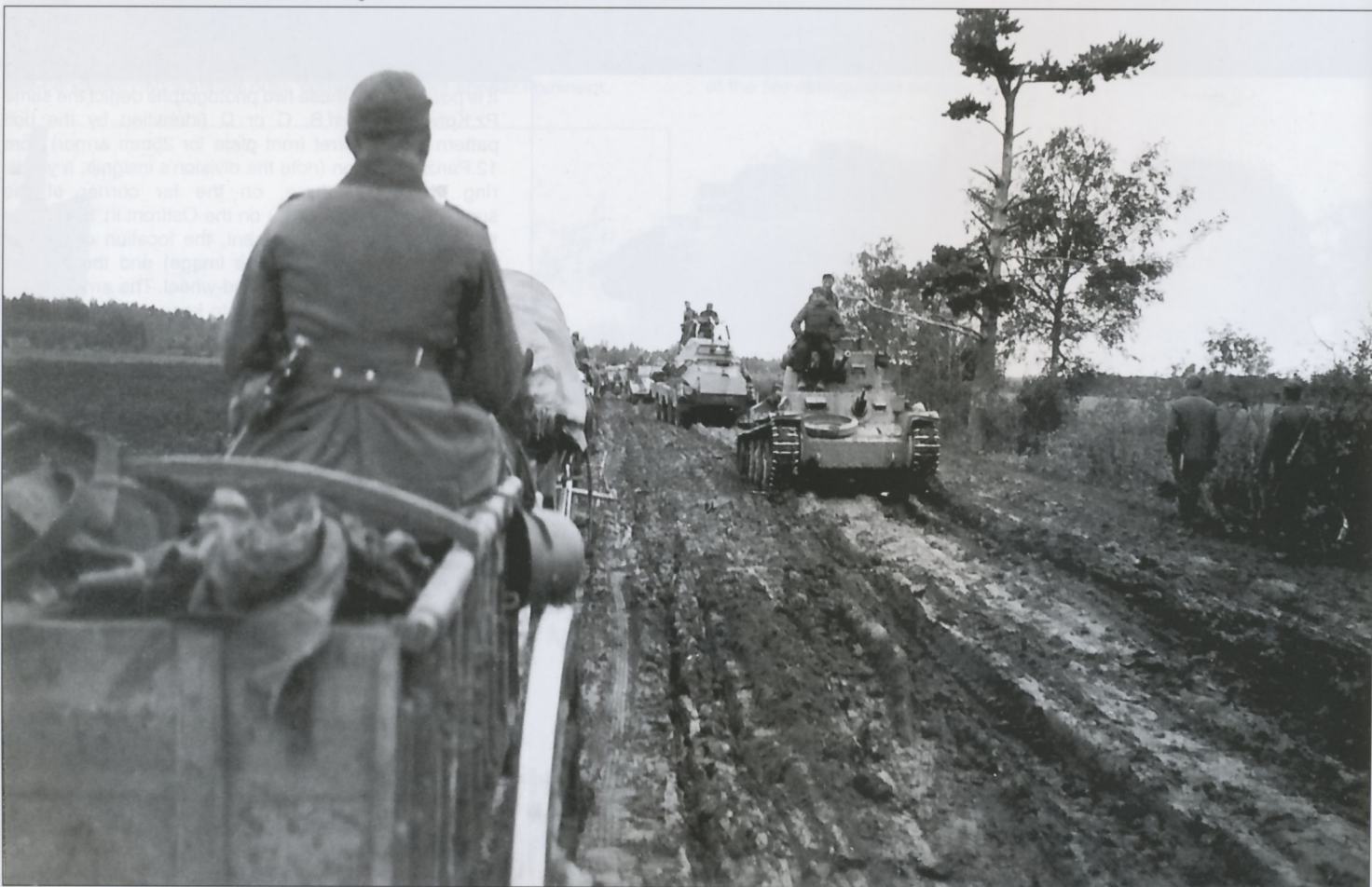
A thoroughly dust-covered Pz.Kpfw.38(t) Ausf. B, C or D, followed by a schwerer Panzerspähwagen (8-Rad) Sd.Kfz.231, leads a column of wheeled vehicles through the mud of a "road" on the Ostfront. The Panzer is identified as an Ausf. B, C or D by the stepped front plate on the superstructure; note the unusual stowage of a road-wheel on the glacis plate.
