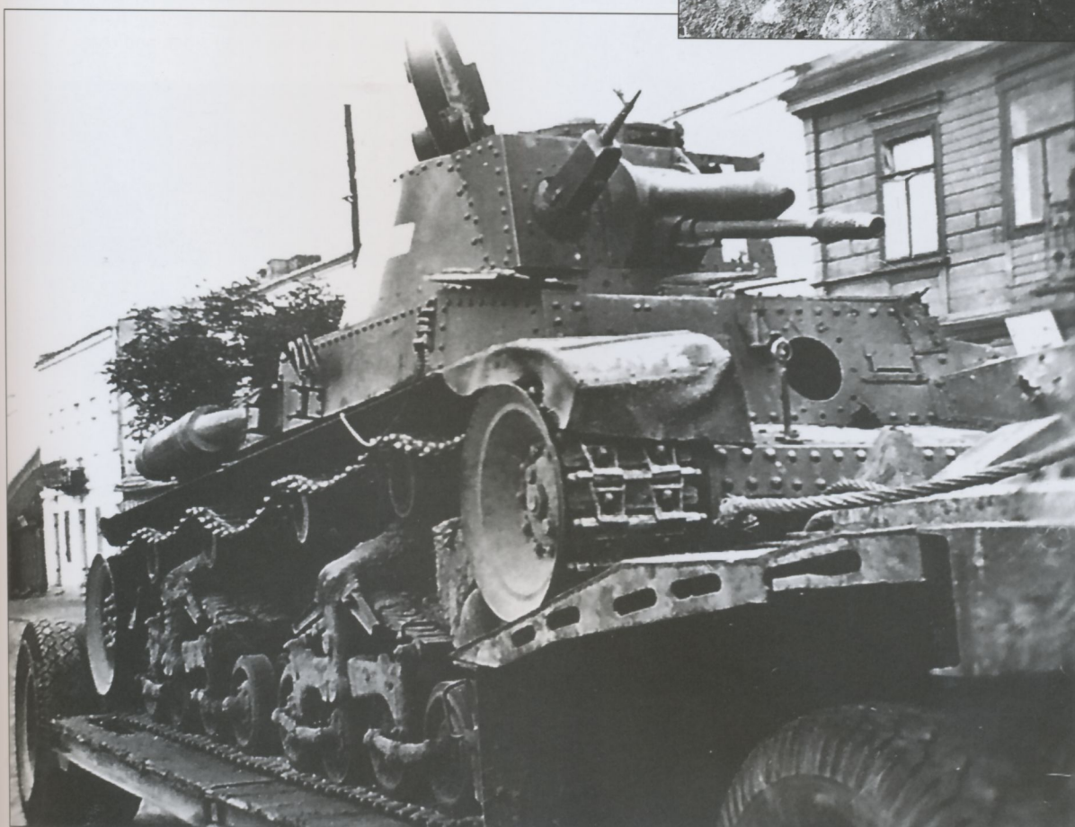
This damaged Panzerkampfwagen (3.7cm) L.T.Sk.35 sits upon a Sd.Ah.115 trailer as it is hauled to workshops for repair. Note the damage to the far track-guard as well as the loss of the mount for the radio operator's 7.92mm MG37(t). Aside from the usual Balkenkreuze national insignia seen on all vertical surfaces of the turret, the three-digit Tac number, 221, is seen on the typical rhomboid plate on the near-side track-guard.
