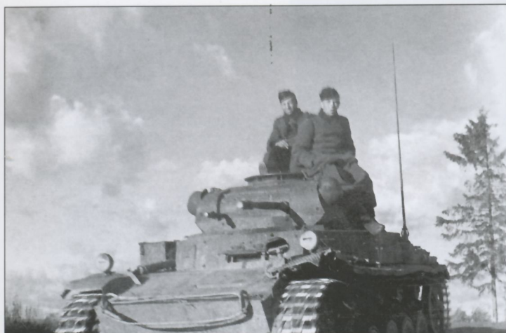
This Pz.Kpfw.II Ausf.A, B or C has been retro-fitted with the commander's cupola that included all around vision using periscopes set about the rim; instead of large split hatch lids, it now has a smaller single circular lid. Other modifications include Zusatzpanzer (appliqué armor panels) on the superstructure front and the turret front and Vorpanzer (spaced armor) on the bow. The slightly mangled port-side track-guard has a Notek black-out driving head-lamp mounted to it; this would be accompanied by a convoy distance-keeping tail-lamp, unseen at this angle.
