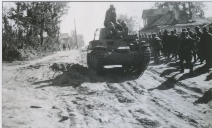
Perched atop his cupola's hatch lid, this commander of a Pz.Kpfw.38(t) Ausf.E or F (note the superstructure front plate's rivet pattern) takes in the sunny summer weather on the Ostfront. The Panzer has been fitted with a typical stowage locker on the track-guard and the crew has also hung their steel helmets on the turret side wall. Most models of the Pz.Kpfw.38(t) had small eyelets attached to various rivet heads located on the turret and superstructure; these had wire or rope threaded through them to which gear (or camouflage material) could be affixed.
