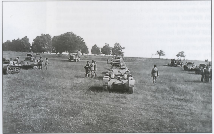
An entire Panzer-Kompanie is lined up on Zug (platoon) columns while on an exercise. The lead vehicle in each column is a Fahrschulpanzer, while those that follow are Pz.Kpfw.I Ausf.Bs. In addition, each column is accompanied by a tactical transport truck, which would carry various consumable items for both Panzer and crewmen.
