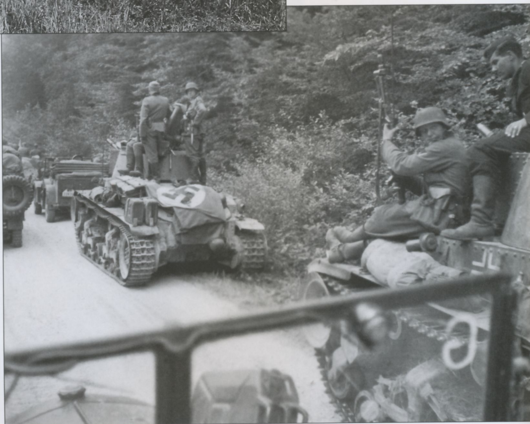
Although difficult to place with any certainty, this Pz.Kpfw.35(t) is probably seen during the French Campaign of 1940. Note the additional rack on the engine deck for 20-liter jerrycans and the rhomboid plate with a white Tac number, 212, just below the rack. The rear hull plate features a black/white Balkenkreuz national insignia, while the Tac numbers are also repeated on the turret sides and rear.
