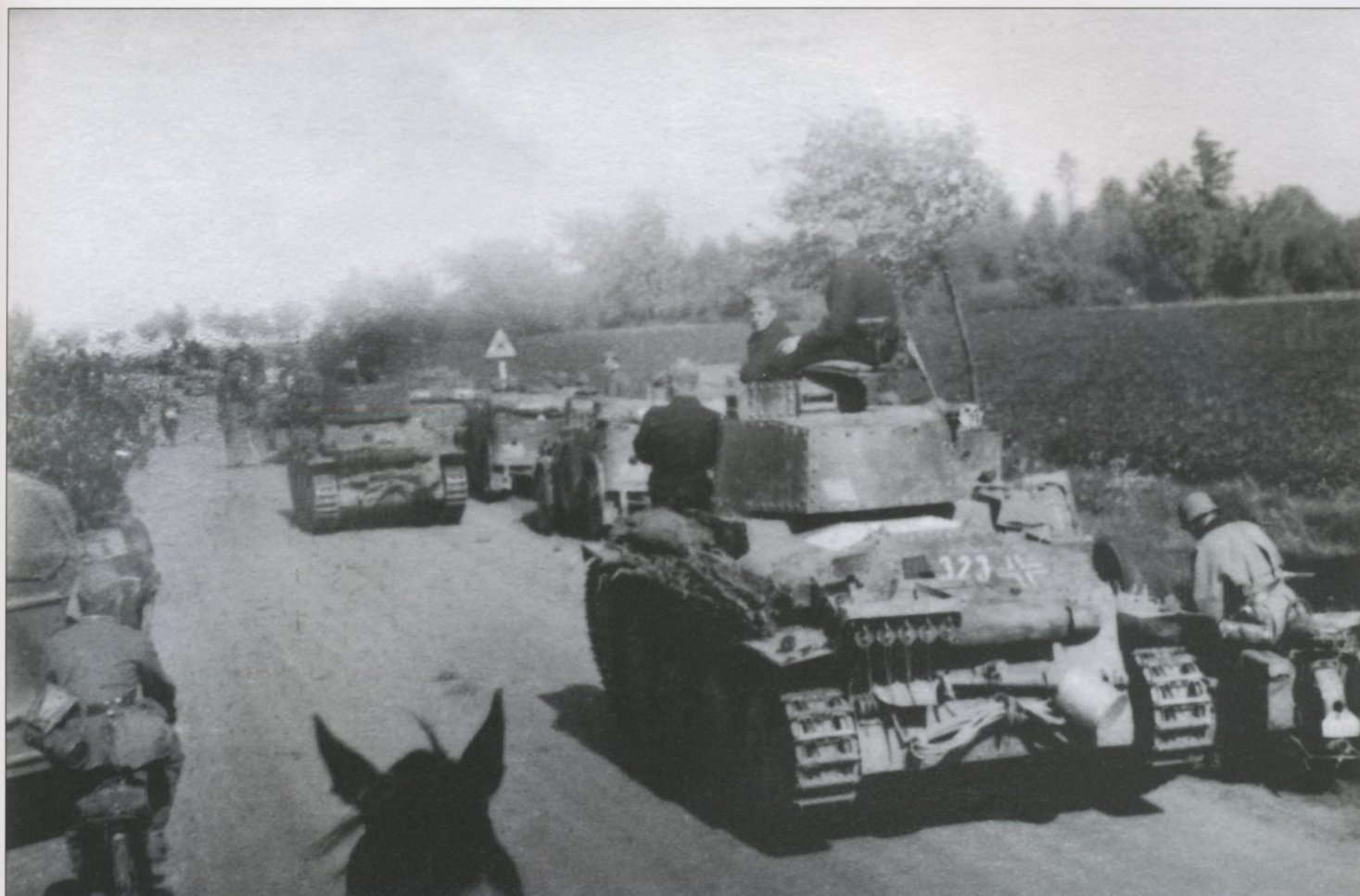
This Pz.Kpfw.38(t) Ausf.B, C or D shows some interesting markings, such as a rhomboid shape painted on the turret rear wall, a three-digit Tac number, 323, on a plate attached to the engine deck, and a white-outline Balkenkreuz beside it. Many units modified tool stowage arrangements, as seen here; note that the shovel and tow cable, normally seen on the superstructure side plate has been moved to the rear hull plate. The track-guards have been fitted with bundles of fascines as well as various stowage lockers, while a five-cell Nebelkerzenabwurfvorrichtung (rack to deploy smoke candles) has been fitted over the exhaust muffler.
