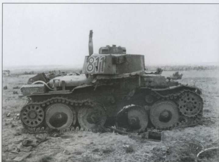
This burned-out 8.Kompanie Pz.Kpfw.38(t) Ausf. B, C or D has seen better days! The turret sports large three-digit Tac numbers, 811 on the side walls; the rear Tac number is painted on a field-applied Gepäckkasten (baggage bin). The perforated stowage locker seen on the track-guards has been re-located aft; just forward of that is what is probably a rack for a 20-liter jerry can. A Notek black-out driving head-lamp has been fitted to the front end of the port side track-guard; thus it is likely that this Panzer was destroyed on the Ostfront.
