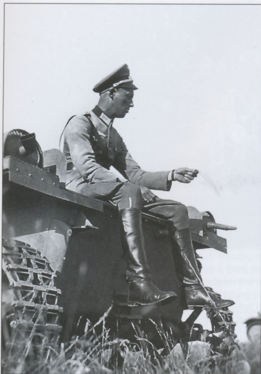
A German Heer (army) officer takes a break while perched on the engine deck of a Pz.Kpfw.I Ausf.A. This unusual view shows the curvature of the lower section of the hull rear plate, the trailer hitch with pin, as well as the bolted mounts for a tow cable. Other visible details include the rear sections of the track-guards as well as the exhaust muffler fish-tails.
