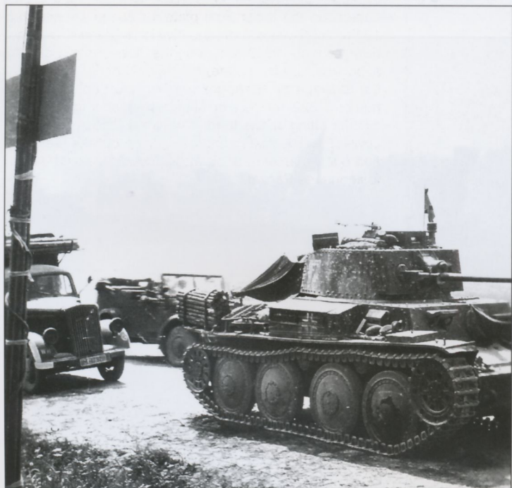
This mud-spattered Pz.Kpfw.38(t) Ausf. E, F or G leads a group of wheeled vehicles on a road, possibly during the opening phases of Operation Barbarossa. The light field car is a Stoewer or BMW, while the other vehicle is an Opel Blitz 3-ton truck. The Panzer has a stowage locker as well as a rack holding a bundle of wired-together saplings on the near track-guard; the latter was used to help negotiate soft ground. A Nazi flag, used as an aerial recognition device is hung, tent-like over the engine deck, while a smaller pennant is fixed to a small staff next to the commander's cupola.
