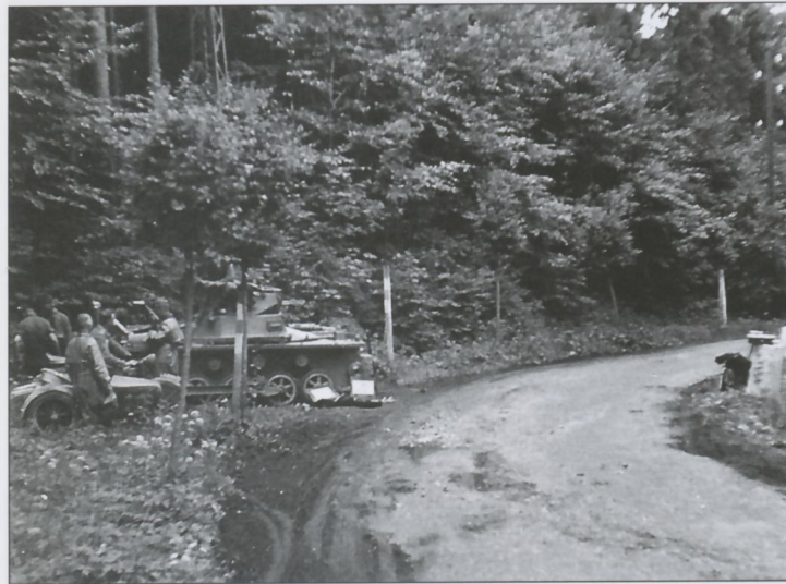
This Pz.Kpfw.I Ausf.A has pulled off to the side next to a bend in the road, apparently with transmission or final drive problems. Note that the tracks have been un-pinned and the drive sprocket has been removed. The white shapes on the ground at the front of the Panzer appear to be the opened lids of tool boxes.
