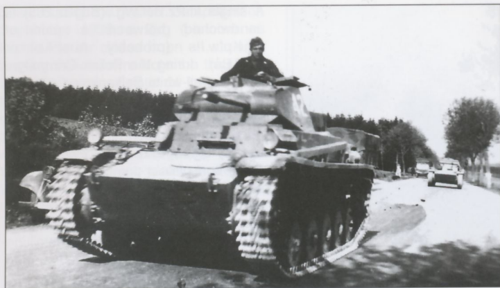
Although difficult to see due to the angle that light strikes the turret side wall, this Pz.Kpfw.II Ausf.A, B or C wears a white, two-digit Tac number, 42. It has some of the post-Polish Campaign modifications to include Zusatzpanzer (appliqué armor panels) on the superstructure front and the turret front, as well as Vorpanzer (spaced armor) on the bow.
